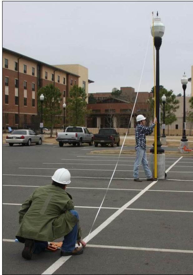
Figure 5. Measuring slope distance with a tape between the top of a light pole and a ground level coordinate identified within a central parking lot on the residential campus of Stephen F. Austin State University, Nacogdoches, Texas.
